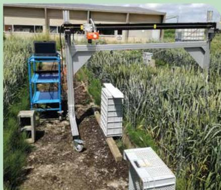
In recent years, the CRA-W has had portable instruments for fluorimetry, spectroscopy and near-infrared imaging to characterise on-site the phenotype of different varieties of beets, potatoes and cereals. In particular, these tools are used to assess the biotic and abiotic stresses on seedlings in greenhouses or plants in the field. Various projects are currently underway at the CRA-W.
