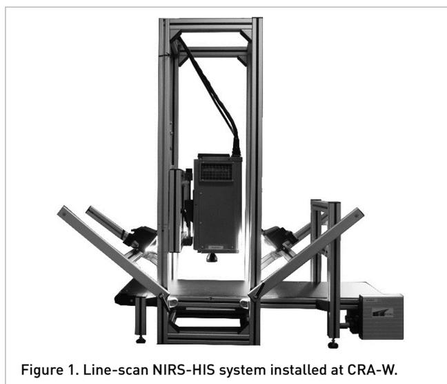
**Figure 1.** Line-scan NIRS-HIS system installed at CRA-W.
