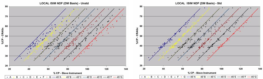
**Figure 3. Scatter plots for seven instruments (A...G) plotted against a master instrument (Y-axis). LOCAL model for NDF before (left) and after (right) standardisation by ISIM.**
