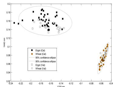
Figure 7: MatrixNIR™: Discrimination Ergot/Wheat based on 2 wavelengths (1220 nm/ 1440 nm)
