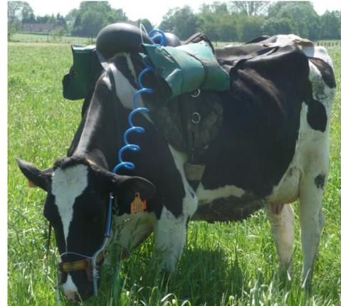
Fig. 2 : Device for collecting a sample of daily enteric CH<sub>4</sub> emissions
