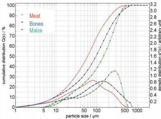
**Figure 4.3.** Overlay of particle size distributions of maize, porcine bones and porcine meat using the cuvette and lens R6 with isopropanol as dispersant. Open circle = meat, square = bones and triangle = maize.
