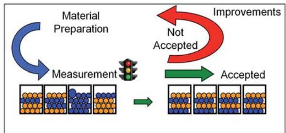
**Figure 4.1.** Schematic illustration of material preparation based on repeated measurements of the heterogeneity of a key parameter and improvements in the material processing. The improved homogeneity is illustrated among the samples to the right with no between bottle heterogeneity.
