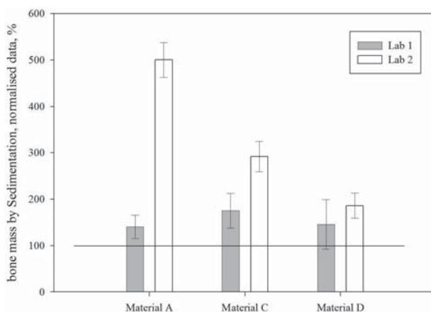
**Figure 4.4.** Results for Phase-2 samples using sedimentation alone. Material B could not be characterised using sedimentation as it contains no bone. The result on the Y-axis is normalised to the added bone mass, target is 100%. The error bars are relative standard deviation for n = 10.
