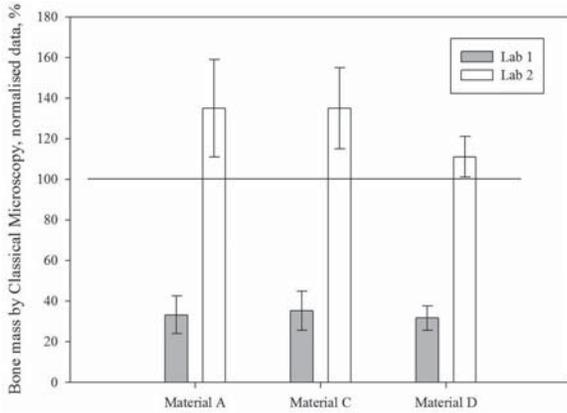
**Figure 4.5.** Results for Phase-2 samples using optical microscopy on the sediment. Material B could not be characterised using sedimentation as it contains no bone. The result on the Y-axis is normalised to the added bone mass, target is 100. The error bars are relative standard deviation for n = 10.
