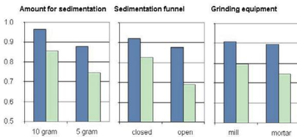
**Figure 5.2.** Bar diagrams of the effect of changing parameters in the microscopic method. Specificity (effect of false positives, dark bars) and sensitivity (effect of false negatives, light bars) is expressed on the y-axis. Source: Raw data of the STRATFEED validation study (Holst et al., 2005).
