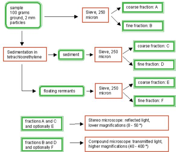
**Figure 5.1.** Outline of the basic steps of the method for microscopic detection of animal proteins in animal feeds. Several recommendations to the basic protocol are included. Source: van Raamsdonk et al., 2004.
