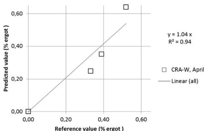
**Fig. 3** Results of the analysis of samples in set A. Correlation between the reference values determined by the official method and the predicted values using the BurgerMetrics NIR hyperspectral instrument
