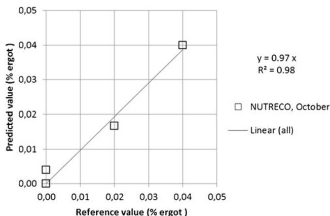
**Fig. 5** Results of the analysis of samples in set B. Correlation between the reference values determined by the official method and the predicted values using the Sisuchema NIR hyperspectral instrument
