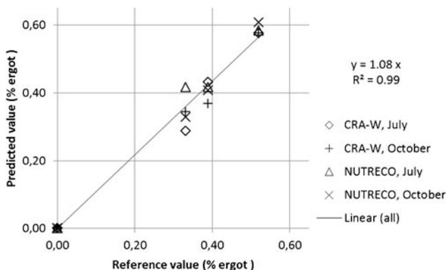
**Fig. 4** Results of the analysis of samples in set A. Comparison of the analysis performed at two locations and over two time periods. Correlation between the reference values determined by the official method and the predicted values using the Sisuchema NIR hyperspectral instrument
