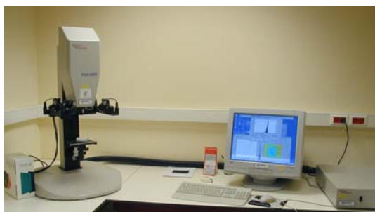
Figure 1: Camera MATRIX NIR installed at CRAGx.
