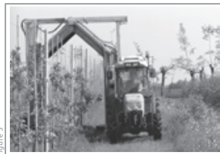
Figure 3 Spray tunnel with six small tanks (each containing a different product mixture), one large rinsing tank and one large mixture recovery tank (experimental prototype).
