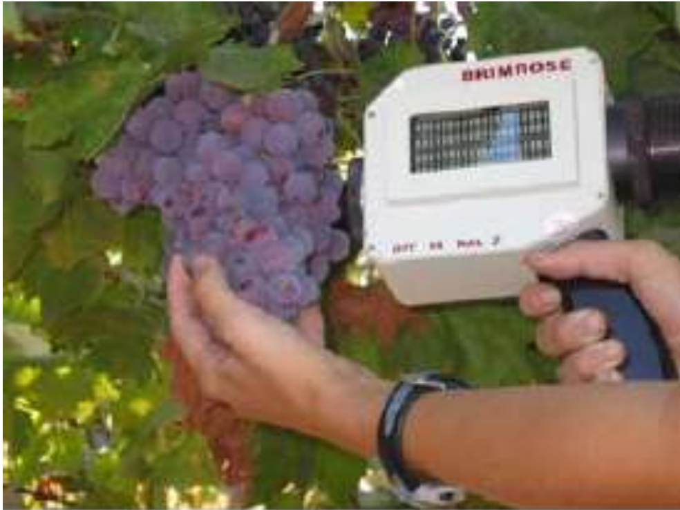
Figure # 1. NIR Hand-held Analyzer is taking readings for Brix, pH, TA in vineyard without removing it from vine
