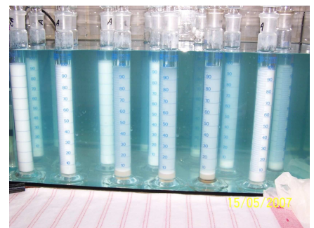
Testing the physico-chemical properties (emulsion stability test) of obsolete FAO pesticide stocks in Africa
