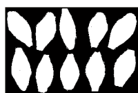
Mask of the image of 10 barley kernels used to calculate the mean spectrum of each barley kernel
