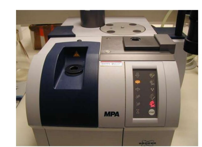
Figure 1: MatrixNIR<sup>TM</sup> Chemical Imaging System instrument characteristics and Bruker MPA instrument
