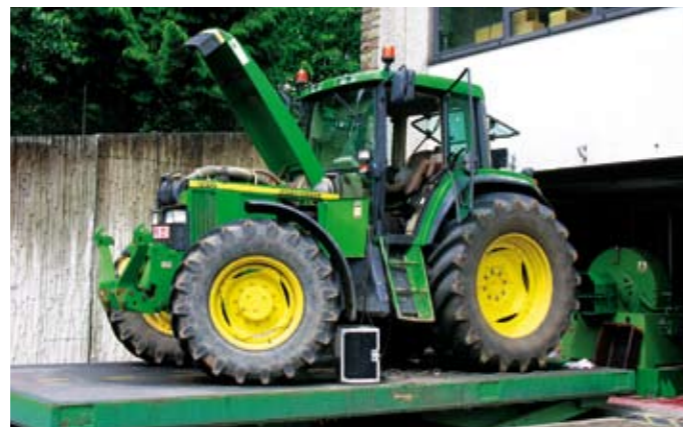
View of test bench and setting up a tractor test.
