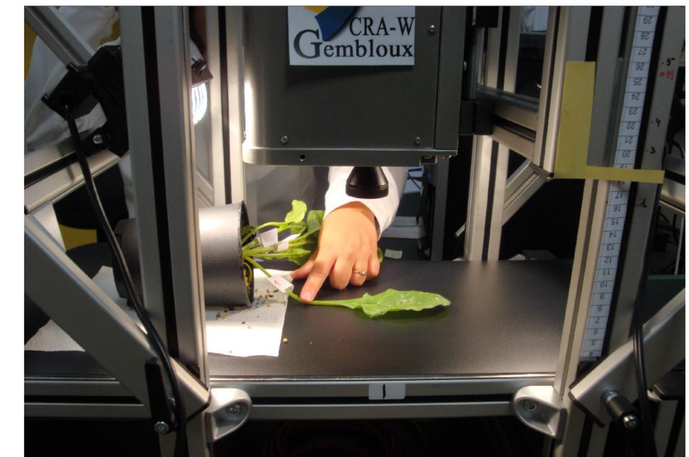
Figure 2: Image acquisition of sugar beet leaves using a line scan hyperspectral imaging system instrument.
