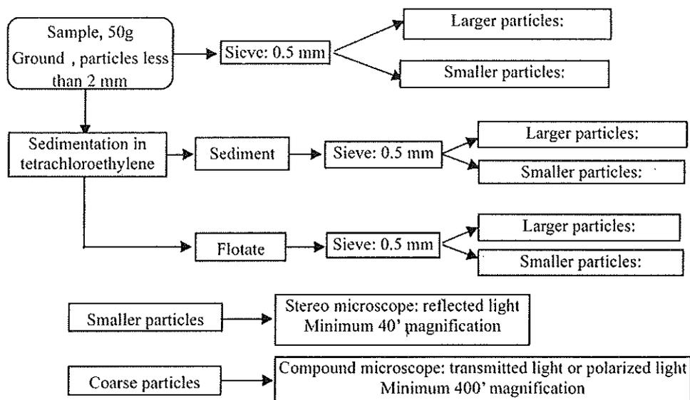
Fig. 1. Analysis procedure for microscopic detection.
