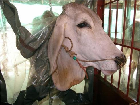
First developed in 2005, after the Japanese 'face mask system' was found to be unsuitable for the climatic and feeding conditions particular to Thailand, the Hood is used to estimate the energy balance in the cattle. The Hood is a respiration trial system using a ventilated flow-through method and comprises five components: (a) a digestion trial pen, (b) head cage, (c) gas sampling and analysis unit, (d) behaviour monitoring unit, and (e) data acquisition and processing unit.
