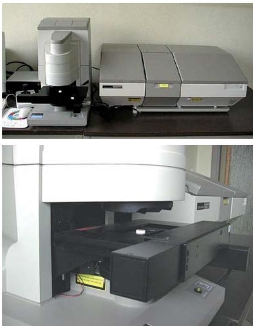
Figure 8.1 - NIR microscope
