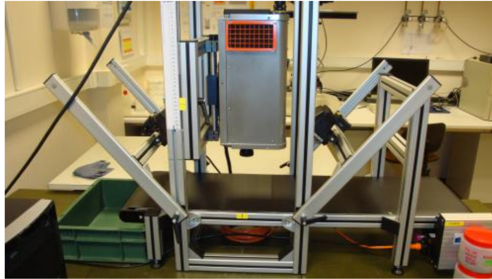
Figure 1 : NIR line scan (pushbroom) hyperspectral camera equipped with conveyor belt (Burgermetrics) .
