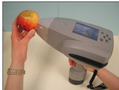
Figure 13 : PHAZIR (Polychromix, Inc.) 1000 – 1800 nm (NIR uniquement)
