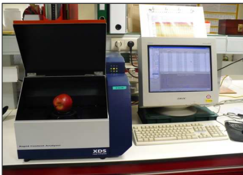
Figure 12 XDS (FOSS NIRSystems, Inc.) 400 – 2500 nm (VIS et NIR)
