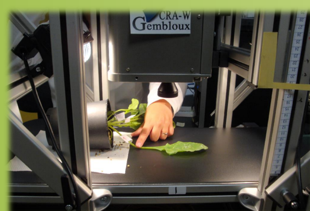
Figure 1: Image acquisition of sugar beet leaves using a line scan hyperspectral imaging system instrument.
