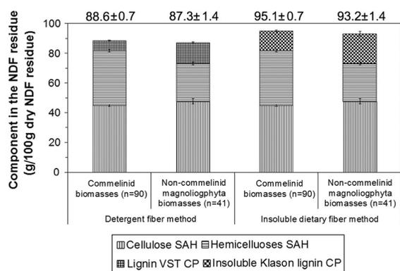
**Fig. 4** Mass balance (mean  $\pm$  confidence interval of the mean) of neutral detergent fiber residue. Error bars correspond to confidence interval of the mean, n to the number of analyzed samples. CP Corrected for protein-like compounds. VST Van Soest
