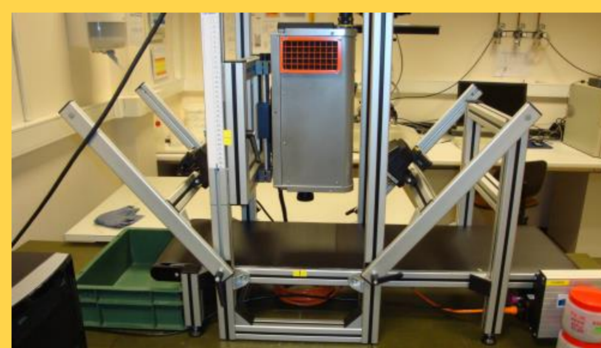
Hyperspectral NIR imaging system with conveyor belt (Burgermetrics)
