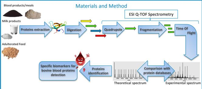
Figure 2: Tandem mass-spectrometry for the selection of bovine blood biomarkers
