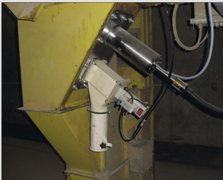
Figure 1. On-line NIR probe and sampling device installed at a feed reception stage (courtesy of Provimi, France. Q-Saffe European project).
