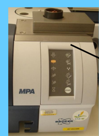
Bruker MPA: bulk sample presentation accessory: ring cup
