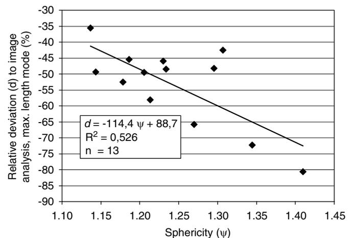
Fig. 8. Linear regression analysis for the relative deviations ( $d$ ) of the median values by horizontal screening (“Horizontal 1”) from image analysis results as a function of the mean particle’s sphericity ( $\psi$ ). Image analysis results gained in “max. length” mode measured with the conventional fuel samples.
