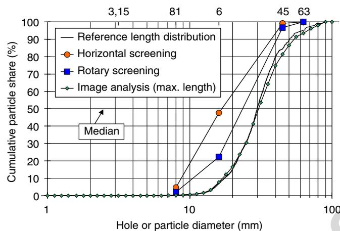
Fig. 7. Cumulative particle size distribution, examples for different testing methods applied on the standard wood chips sample.
