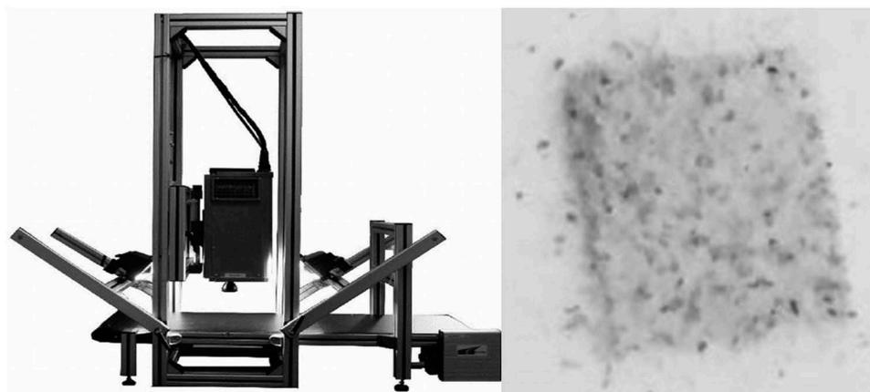
**Figure 2.** Burgermetrics near-infrared (NIR) hyperspectral imaging system and cereal flour adulterated with ergot on spectralon.
