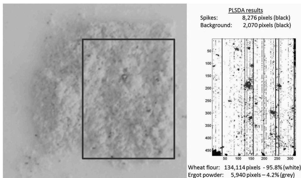
**Figure 3.** (left) RGB picture and (right) predicted near-infrared (NIR) hyperspectral image showing spikes (black line), background (black), ergot particles (grey) in a wheat flour (white) sample adulterated with 5% ergot powder.
