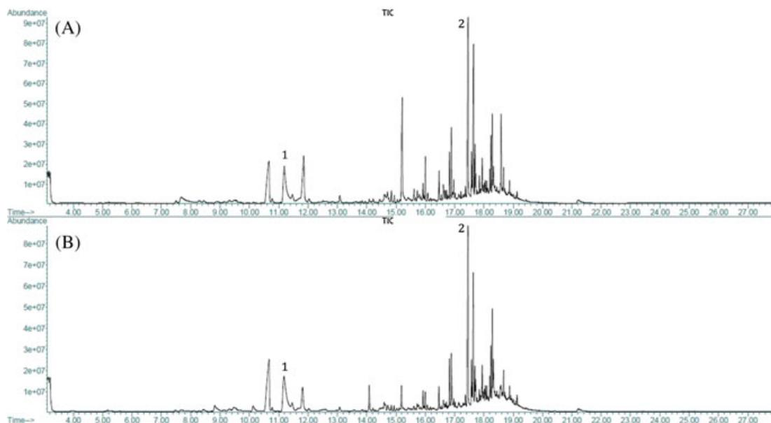
**FIGURE 3** Total ion chromatogram (TIC) for (A) whole profile of blank test performed on growing medium and (B) whole profile of 28-day-old plantlets of *Brassica napus* L. var. *Es Astrid* volatiles. Peak identification: 1: *n*-butyl benzene internal standard (IS) not used, 2: octylbenzene (IS) [Colour figure can be viewed at [wileyonlinelibrary.com](http://wileyonlinelibrary.com)]
