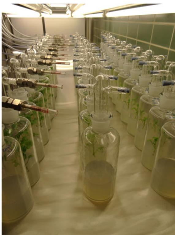
**FIGURE 2** Picture of the high-throughput dynamic headspace sampling technique using Tenax® TA cartridges connected to the cuvette system with swageloks® stainless steel links for a sampling time of 24 h [Colour figure can be viewed at [wileyonlinelibrary.com](http://wileyonlinelibrary.com)]
