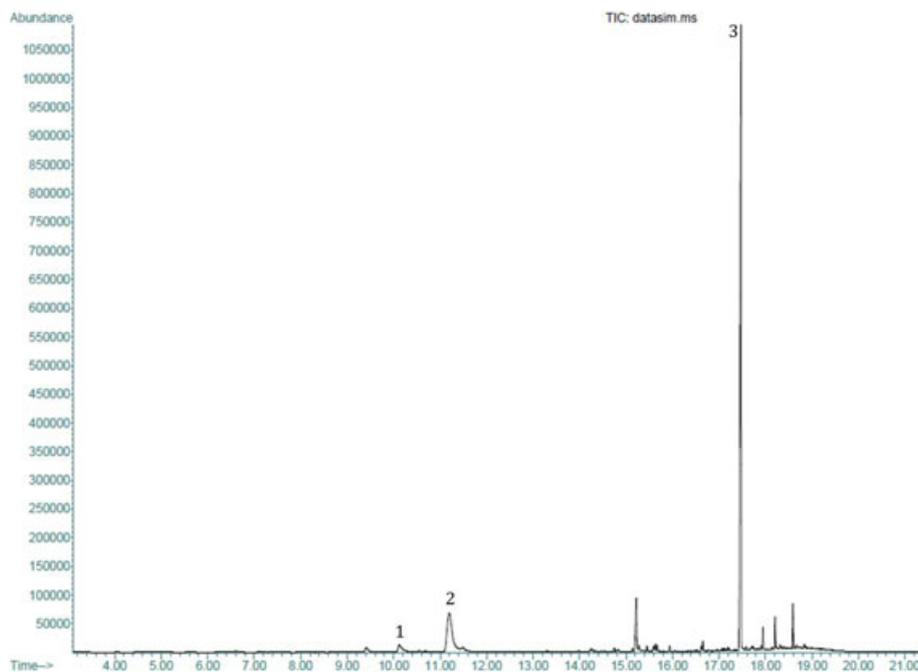
**FIGURE 4** Typical chromatogram of growing medium using selected ion monitoring (SIM) mode. Peak identification: 1: limonene, 2: *n*-butyl benzene internal standard (IS) not used, 3: octylbenzene (IS) [Colour figure can be viewed at [wileyonlinelibrary.com](http://wileyonlinelibrary.com)]
