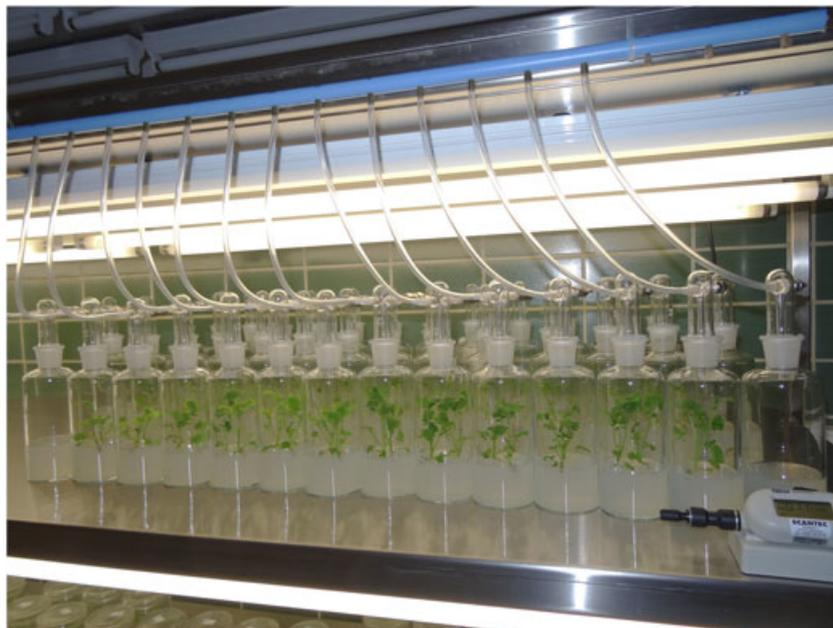
**FIGURE 1** Picture of the laboratory glass chamber system allowing the *in vitro* growth of *Brassica napus* L. plantlets and the trapping of VOCs under cadmium-related abiotic stress [Colour figure can be viewed at [wileyonlinelibrary.com](http://wileyonlinelibrary.com)]
