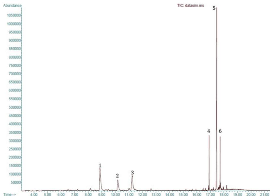
**FIGURE 5** Typical chromatogram of 28-day-old plantlets of *Brassica napus* L. var. *Es Astrid* using selected ion monitoring (SIM) mode. Peak identification: 1: myrcene, 2: limonene, 3: *n*-butyl benzene internal standard (IS) not used, 4:  $\beta$ -elemene, 5: octylbenzene (IS), 6: (E,E)- $\alpha$ -farnesene [Colour figure can be viewed at [wileyonlinelibrary.com](http://wileyonlinelibrary.com)]
