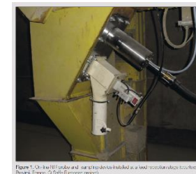
Figure 1. On-line NIR sensor and imaging system installed in a seed processing plant (courtesy of Provimi, France). © 2010 European Society of Plant Pathology
