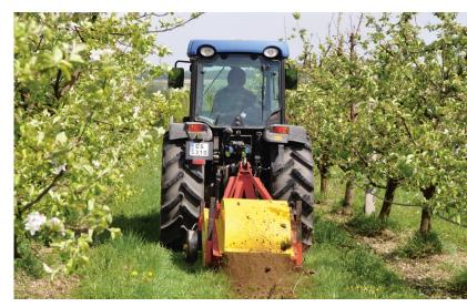
The recommended width for flower strips is equal to the inner distance between the tractor wheels plus 10 cm, resulting in a 5 to 10 cm overlap into the tractor track at each wheel. Flower strip width also depends on the available machinery for soil preparation and mulching.
