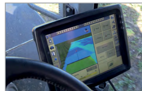
Tractor spreading fertiliser according to a variable rate application map made in CropSAT.
