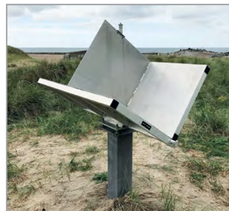
Corner reflector developed by DTU Space & Agency for Data Supply and Efficiency and manufactured by Lemvig Utility. Reflectors serve to link height variations in EO data to the Danish datum network (Photo by kind permission of Mr. Karsten Vogensen).
