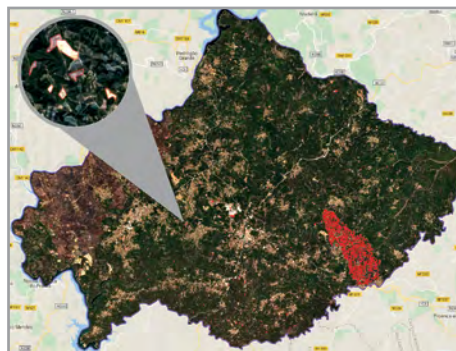
The red polygons show automated change detections in region of Sertã, Portugal (large: forest fire, small: disease outbreaks).
