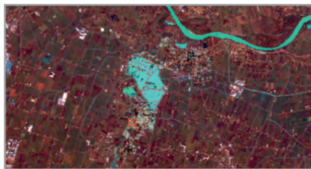
Italy - Reggione Emilia 2017, multispectral image (Sentinel) showing flooded areas, in light blue, near Lentigione town due to Enza river flooding. Credit: Contains modified Copernicus Sentinel data [2017]
