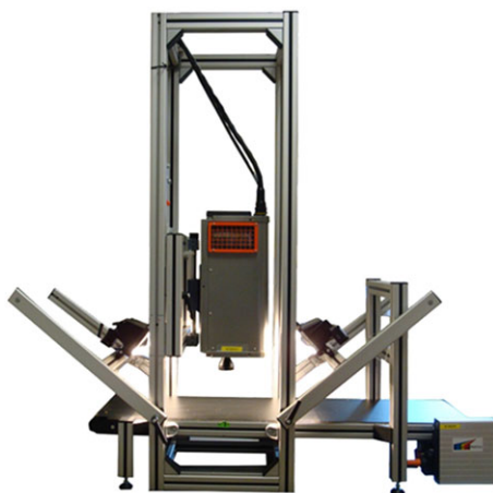
FIGURE 2 Near-infrared (NIR) hyperspectral imaging system installed at the Walloon Agricultural Research Center, Belgium (BurgerMetrics SIA, Riga, Latvia)
