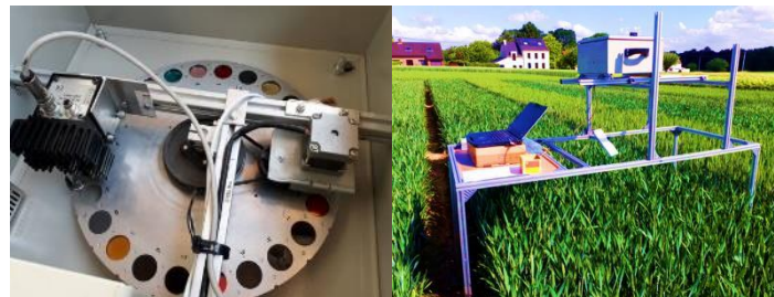
Figure 1: Proximal multispectral acquisition system. On the left, the camera and the motorised filter wheel. On the right, the full platform supporting the acquisition system.
