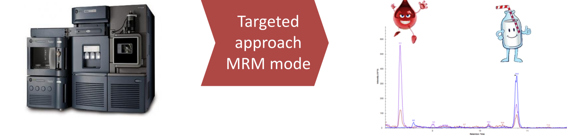
Figure 1: Proteins extracted from adulterated samples were digested. Extracts were then purified by using one type of SPE cartridge and analysed by LC-MS/MS for the detection of bovine haemoglobin, bovine casein and bovine beta-lactoglobulin peptides.
