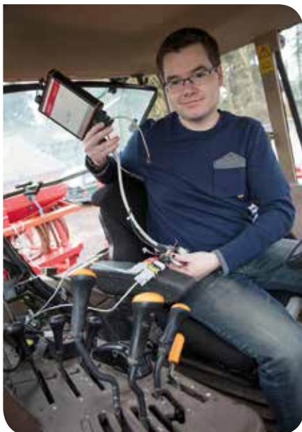
Image legend: A datalogger the size of a DVD box can autonomously record all data relating to a tractor over several months.
