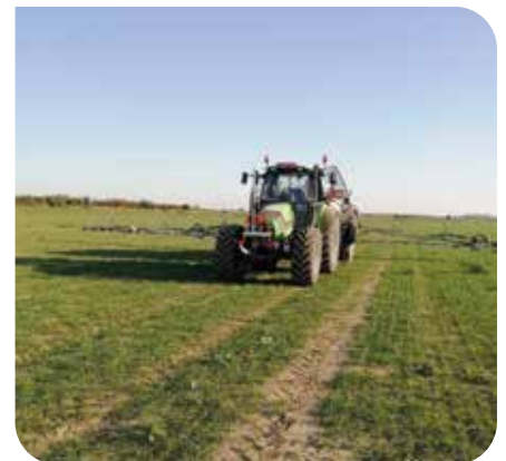
Sprayer equipped with on-board sensors to enable spot-spraying
