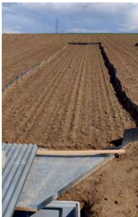
Plot for measuring run-off, sediment and pesticide flows, used in the Intell'eau project trials
