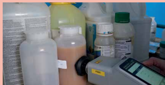
Measurement of a pesticide formulation using a portable Raman device
