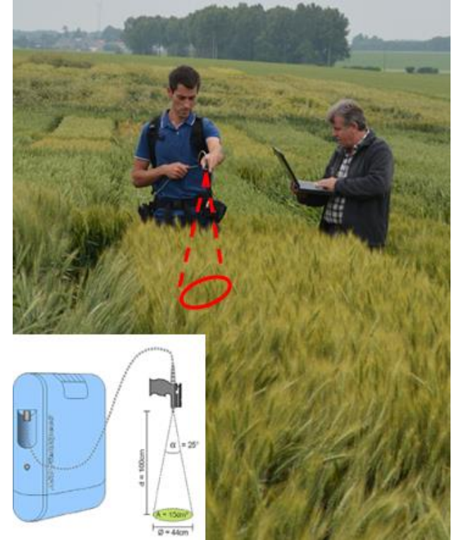
Reflectance data acquired using the ASD FieldSpec 4 equipped with the pistol grip
