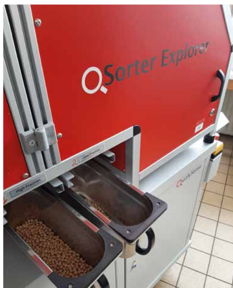
Seed-to-seed optical sorting of peas with QSorter Explorer (QualySense, CH)
