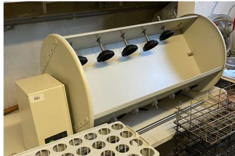
Blender: Heidolph Reax 20 mixer 3 rpm
